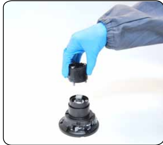
7. Remove the self-tailing arm support n°2 and slide out the bushing
