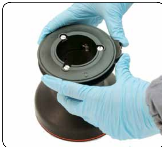
If the jaws have been disassembled, insert peeler between the two jaws, taking care that the letters TOP on the peeler are facing upwards.
