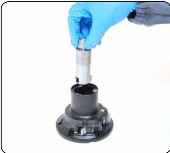
8. Slide out the central shaft n°14
