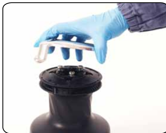
4. Remove the self-tailing arm n°18 by rotating and lifting it.
