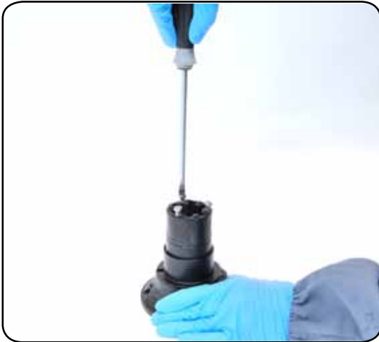
6. Completely unscrew the three screws n°17
