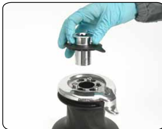
2. Slide off the assy socket n°15 and the cover n°20
