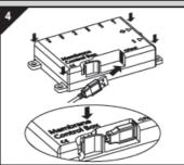
Install the Control Box properly with the included screws.
