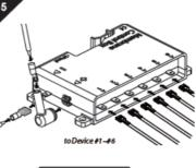
Crimp the DC positive wire (+) with the included round terminal. Pass the wire through the included insulator and connect to the screw terminals. Cover the terminals with the insulator properly. Crimp the DC negative wire (-) with the insulated 0.250" female terminal and insert into the negative quick terminal on Control Box.
