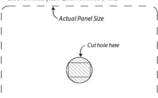
This template is provided to help you install the membrane panel correctly. Cut out template and trace onto the dashboard. Then drill a hole at the shielded area.
