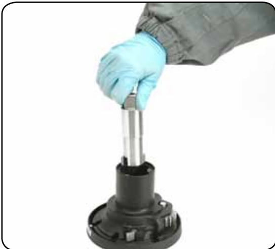
8. Slide out the central shaft n°7
