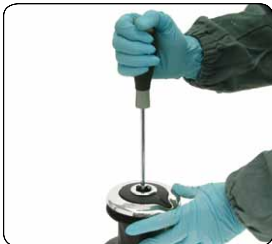
1. Unscrew the central screw ( \approx 2\text{Nm}/18\text{ in-lb} )
