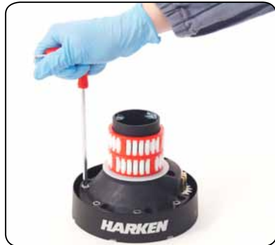
9. Unscrew the 6 hex screws n°16 (8Nm/71 in-lb)
