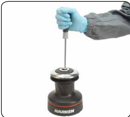
1. Unscrew the central screw ( \approx 2\text{Nm}/18\text{ in-lb} )
