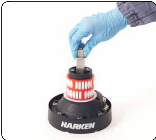
8. Slide out the central shaft n°19
