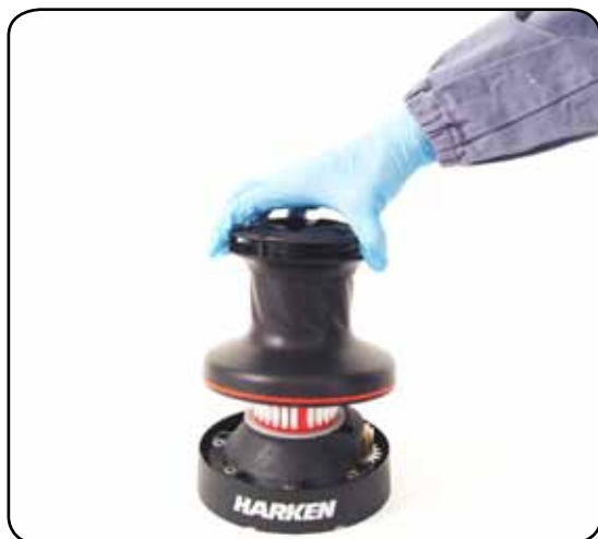
5. Lift off the drum n°22
