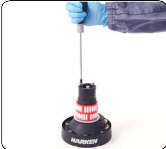
6. Completely unscrew the three screws n°27
