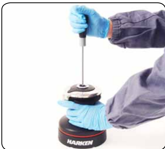
1. Unscrew the central screw ( \approx 2\text{Nm}/18\text{ in-lb} )
