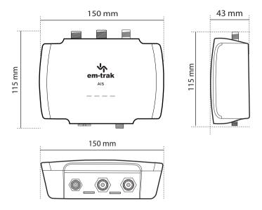
Figure 9 AIS transceiver dimensions
