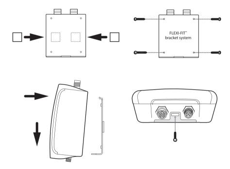
Figure 11 AIS transceiver mounting
