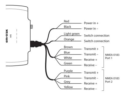
Figure 7 Power and data cable connections
