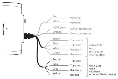
Figure 17 Connecting to your NMEA 0183 sensor
