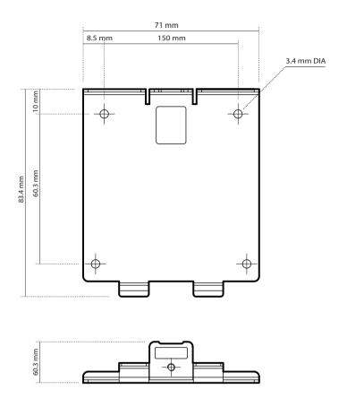
Figure 2 FLEXI-FIT bracket
