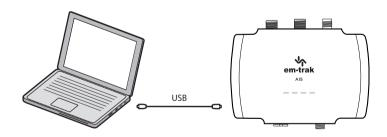
Figure 12 Configuration using your PC
