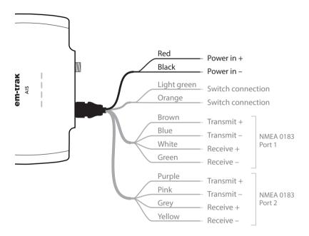
Figure 8 Connecting the power supply
