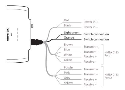
Figure 20 Connecting an external switch
