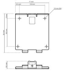
Figure 10 FLEXI-FIT bracket
