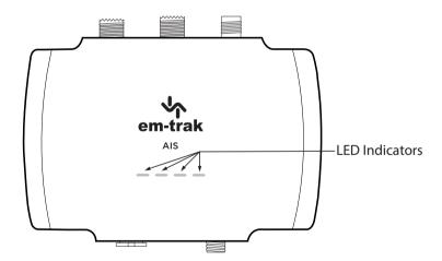
Figure 19 LED indicator location on the AIS transceiver unit
