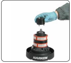
6. Completely unscrew the three screws  $n^{\circ}$  28 and remove the stripper arm support  $n^{\circ}$ 22
