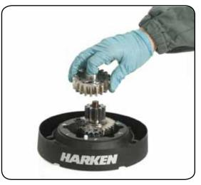
12. Remove the gear  $n^{\circ}10$  and remove the pawls carrier  $n^{\circ}7$ .
