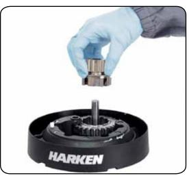
14. Remove the pinion n°11. To facilitate the operation press the spring against the pawl with a blade
