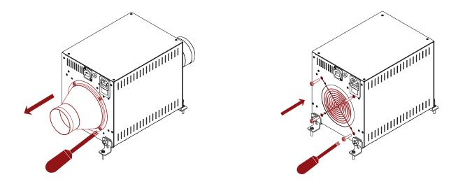
3. Additional air duct components can be added to the heater for distributing hot air. Each of the components reduces total flow rate of hot air. To be sure that the option you choose for the installation of air ducts, is acceptable and will not result in a massive flow rate reduction of hot air or overheating of the heater you have to consider the distribution of the air with different components. Here are shown some examples:
