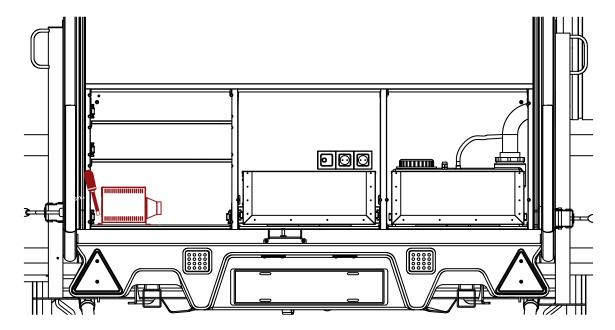
2. Mount the Ø65mm heating pipe on the outtake of the heater. Use two TX 20 self-drilling screws and screw them through the heating pipe and into the holes of the heater's outtake. Use the heat resistant tape with a double layer and cut it. This is how all the connections should be assembled. (Part used: A, D and E)
