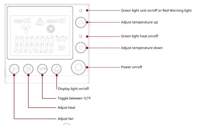
To turn on the unit push the ON/OFF button. The unit will start with the last used setting due to integrated memory function. Push the HEAT button to adjust the watt. The heat button has a rolling action function. This means the button has 5 steps. It will change from 0 to 1 to 2 to 3
