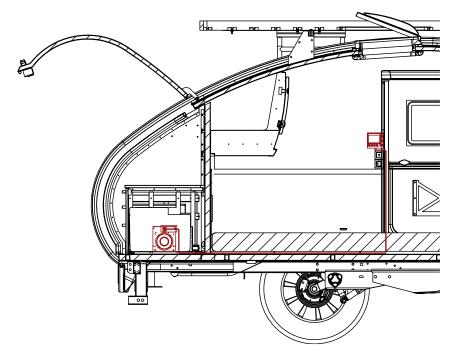
6. Insert the power cord to the heater and plug it into the socket. Please see **step 8** - INSTALLATION GUIDE – GENERAL.
