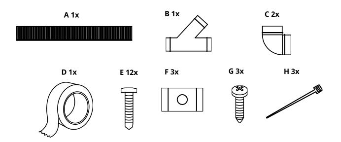
**A:** Ø65mm air heating pipe 1.8m **E:** Self drilling screw TX20 4x25mm
