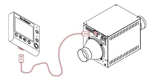
7. The Additional Temperature Sensor can be inserted if you want to adjust the Electric Air Heaters temperature on a different spot then the LCD Display or if you want to use the Electric Air Heater without display and only through the APP (Please see section APPLICATION.) The Additional Temperature Sensor has higher priority than the temperature sensor in the LCD Display. (Part used: H)
