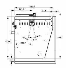
Fuel Type: Input Gas Pressure: Rapid Burner Output: Auxiliary Burner Output: Oven Burner Output: Broiler Output: Oven Volume: Electrical Requirement Weight: Warranty: Propane / Butane 30 mbar (4) @ 8500 BTU / 2.5 Kw (each) (1) @ 3400 BTU / 1 Kw 6370 BTU / 1.87 Kw 6800 BTU / 2 Kw 1.3 cu. ft / 36 L 1.5 Volt DC AA Battery 112 lbs (51 Kg) (2) Years
