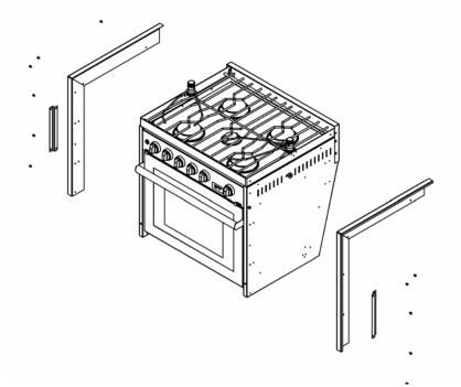
Secure the stove into position by screwing the stove sides to the walls of the cut out. The mounting holes are located as shown. Use #6, 1" stainless steel wood screws (Screws not included)
