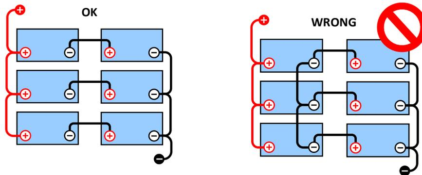
Due to the voltage drop over the positive and the negative cables the midpoint voltage are not identical.
