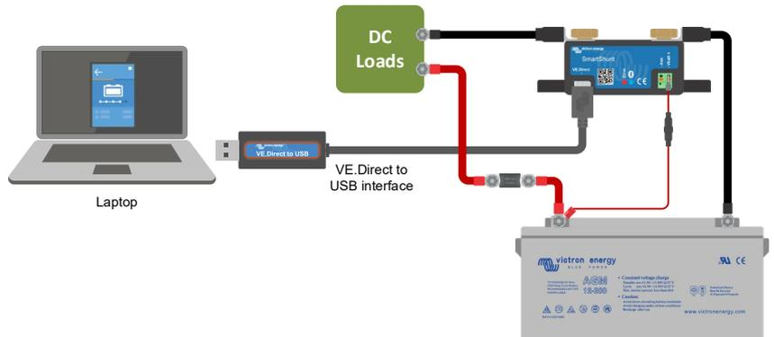
To connect via USB, you will need a “VE.Direct to USB interface”, part number SS030530000. Use this interface to connect the computer to the SmartShunt.
