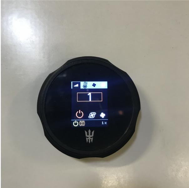
Heater is turned off by selecting power indicator and long press of button.
