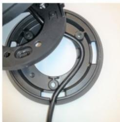
Step 1: Install cable into Wall assembly plate.
