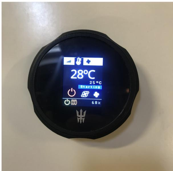
When starting protocol is completed mode indicator "starting" turns off. Selected function is highlighted. When something needs adjustment, select wanted function by turning rotary switch, push button and do wanted changes by rotary switch. Accept changes pushing the button.
