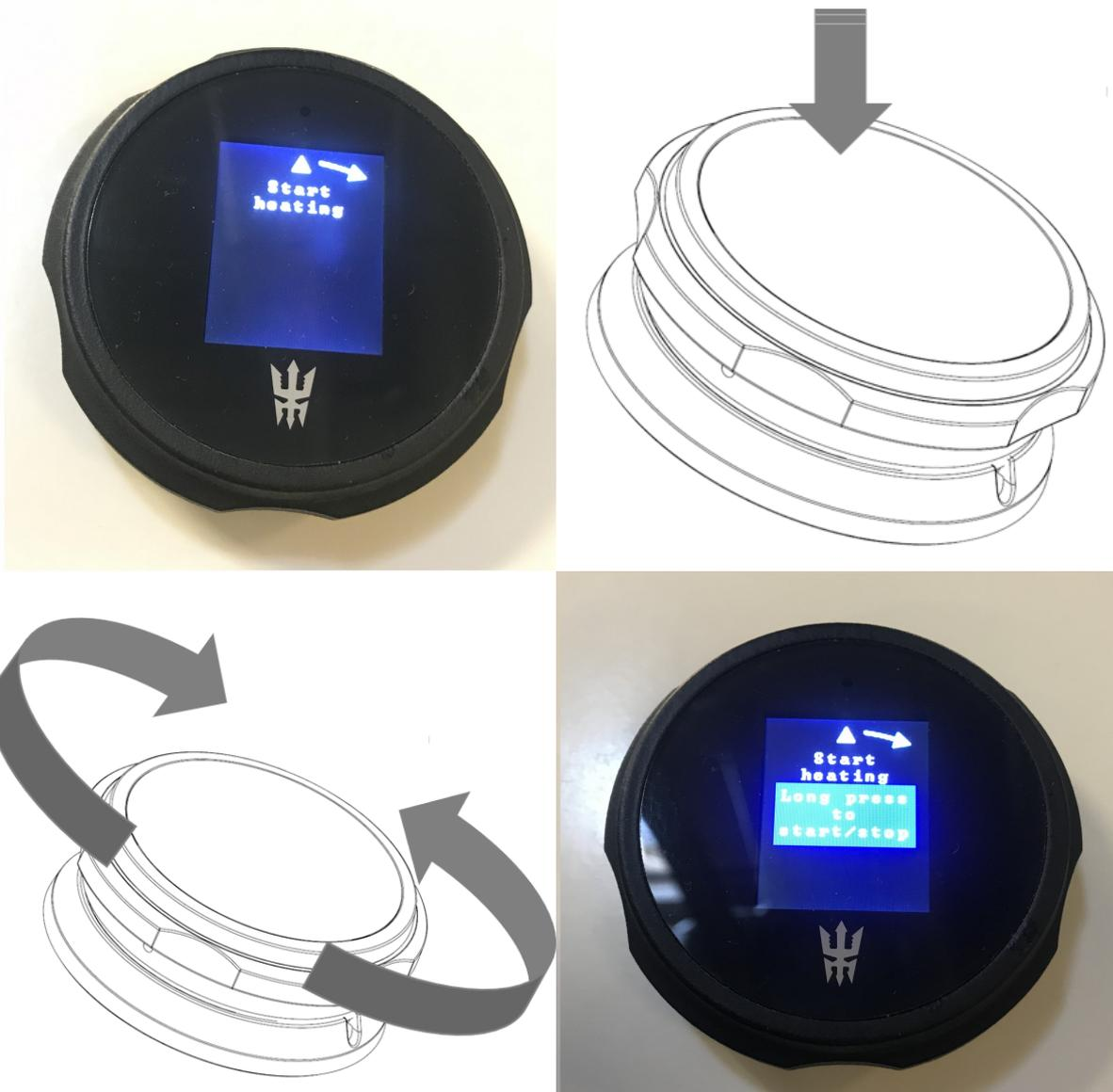
Adjust wanted temperature by rotary switch and accept that with button
